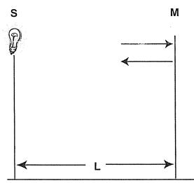
A source of light S and a mirror M facing it, are mounted on a rigid base at distance L. Light travels from S to M and back in a time expressed by T = 2L/C, where C is the speed of light.
