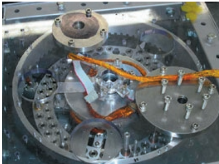
Sample Manipulation Sample (SMS) under construction at Honeybee for 2009 Mars Science Lab (MSL) lander is the crucial component required for delivery of soil/rock samples to on board instruments for detailed scientific analysis.
