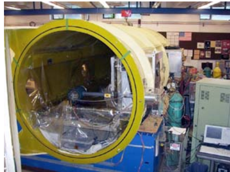
The PHPP Vacuum Vessel (internal view): The PHPP is a 2 meter diameter, 5 meter long fiberglass tank with eight optical access ports. A vacuum level on the order of 10^{-5} torr, for mass flow rates on the order of a few grams per second, is maintained by a set of two 1.3 m diffusion pumps each with a pumping capacity of 95 \text{ m}^3/\text{s} and each is backed by a roots blower (1340 cfm) and a mechanical pump (150 cfm). Ionization gauges allow continuous monitoring of the vacuum. Photo Credit: Steve Krisocki
