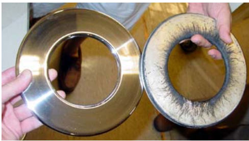
The outer copper ring electrode (the anode) of a thruster before (left) and after (right) intensive firing. The anode has been pitted, scarred, and blackened. Photo Credit: Ken Kremer
