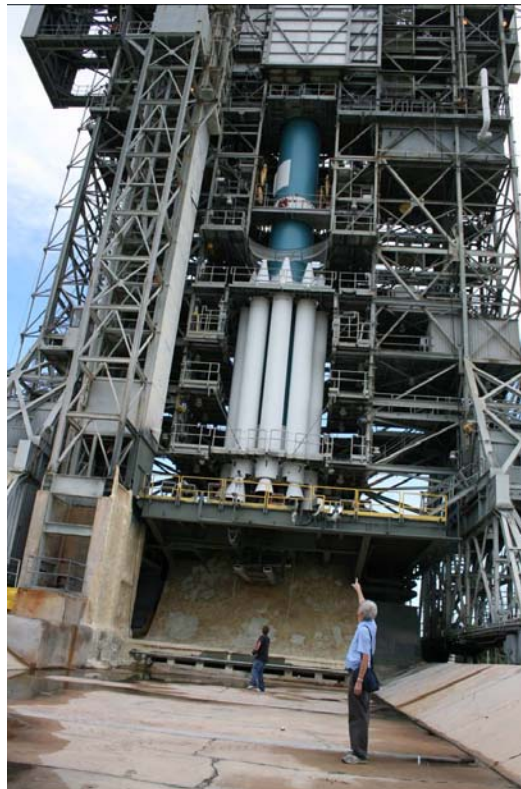
I am gazing at stacked Delta II with solid rocket motors at the launch pad sitting atop flame duct while awaiting ignition of Solid Rocket Motors. Credit: Craig Covault
